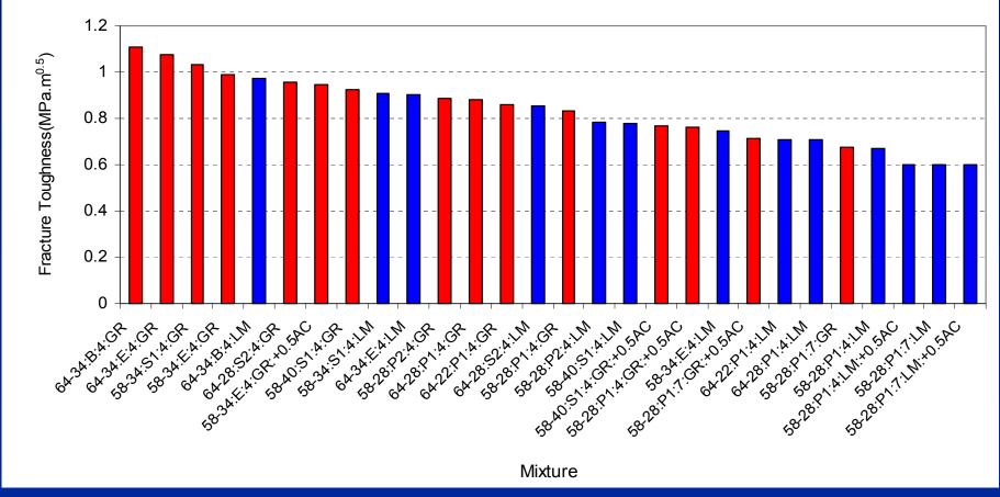
Fracture Toughness Ranking at TM
